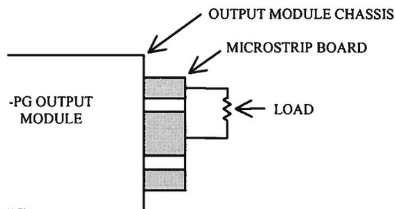
Take care to ensure that during soldering the OUT conductor is not shorted to the chassis. Also, use minimal heat when soldering.
