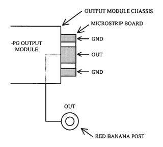
The load should be connected between the OUT and GND terminals using very short leads ( $\leq 2.0$  cm).
