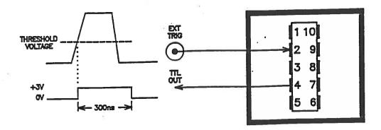
The threshold module acts as a buffer for the EXT TRIG The module accepts trigger inputs of ±0.5V to +40V in amplitude and generates a 300 ns TPL output pulse when the input passes a certain threshold voltage, set by the LEVEL knob on the front panel. When the threshold voltage is negative, the module will trigger when the input is more negative than the threshold. When the threshold voltage is positive, the module will trigger when the input is more positive than the threshold.
