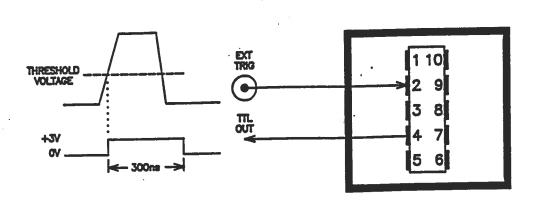
The threshold module acts as a buffer for the EXT TRIG The module accepts trigger inputs of ±0.5V to input. +40V in amplitude and generates a 300 ns TPL output pulse when the input passes a certain threshold voltage, set by the LEVEL knob on the front panel. When the threshold voltage is negative, the module will trigger when the input is more negative than the threshold. When the threshold voltage is positive, the module will trigger when the input is more positive than the threshold.
