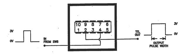
The pulse width module sets the pulse width of the main front panel output. The input is a TTL pulse from one of the two outputs on the clock module, selected by SW5. If the ADVANCE mode is selected, the SYNC pin of the clock module triggers the pulse module. If the DELAY or DOUBLE PULSE mode is selected, the OUT pin of the clock module triggers the pulse module.
