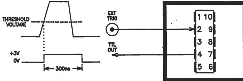
The threshold module acts as a buffer for the EXT TRIG input. The module accepts trigger inputs of +0.5V to +40V in amplitude and generates a 300 ns TTL output pulse when the input passes a certain threshold voltage, set by the LEVEL knob on the front panel. When the threshold voltage is negative, the module will trigger when the input is more negative than the threshold. When the threshold voltage is positive, the module will trigger when the input is more positive than the threshold.
