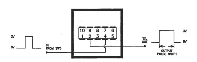
The pulse width module sets the pulse width of the main front panel output. The input is a TTL pulse from one of the two outputs on the clock module, selected by SW5. If the ADVANCE mode is selected, the SYNC pin of the clock module triggers the pulse module. If the DELAY or DOUBLE PULSE mode is selected, the OUT pin of the clock module triggers the pulse module.
