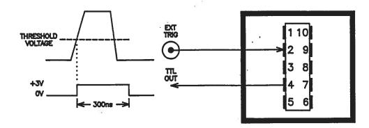
The threshold module acts as a buffer for the EXT TRIG input. The module accepts trigger inputs of +0.5V to +40V in amplitude and generates a 300 ns TTL output pulse when the input passes a certain threshold voltage, set by the LEVEL knob on the front panel. When the threshold voltage is negative, the module will trigger when the input is more negative than the threshold. When the threshold voltage is positive, the module will trigger when the input is more positive than the threshold.
