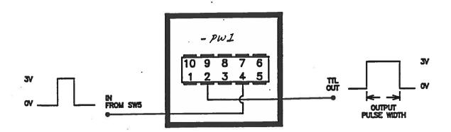
The pulse width module sets the pulse width of the main front panel output. The input is a TTL pulse from one of the two outputs on the clock module, selected by SW5. If the ADVANCE mode is selected, the SYNC pin of the clock module triggers the pulse module. If the DELAY or DOUBLE PULSE mode is selected, the OUT pin of the clock module triggers the pulse module.
