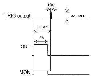
Basic Output Pulses for Delay < 0
