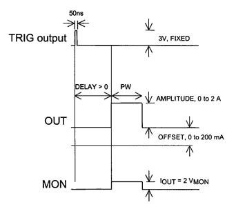
Basic Output Pulses for Delay > 0
