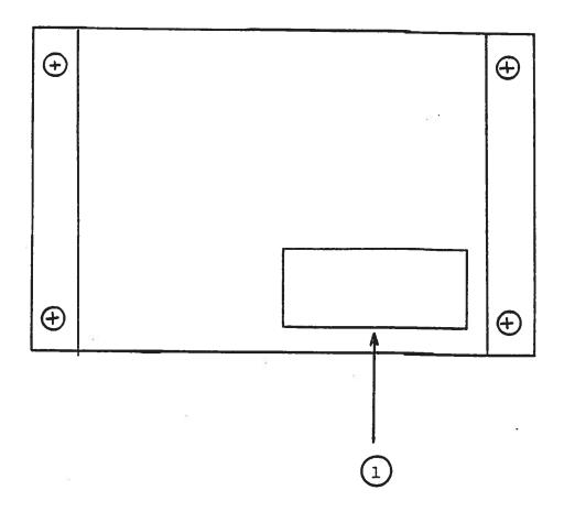
(1) FUSED CONNECTOR, VOLTAGE SELECTOR. The detachable power cord is connected at this point. In addition, the removable cord is adjusted to select the desired input operating voltage. The unit also contains the main power fuse (0.25 A SB).
