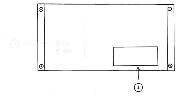
(1) <u>FUSED CONNECTOR, VOLTAGE SELECTOR</u>. The detachable power cord is connected at this point. In addition, the removable cord is adjusted to select the desired input operating voltage. The unit also contains the main power fuse (0.25 A SB).
