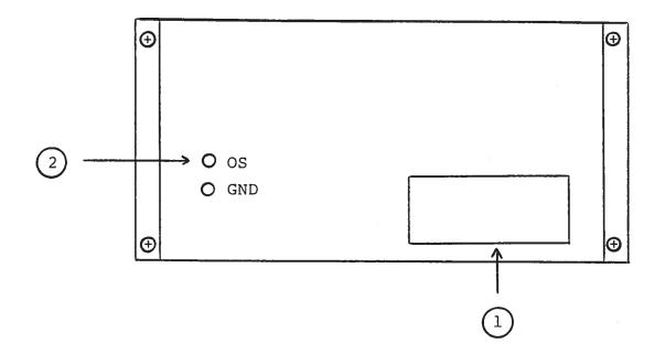
1) FUSED CONNECTOR, VOLTAGE SELECTOR. The detachable power cord is connected at this point. In addition, the removable cord is adjusted to select the desired input operating voltage. The unit also contains the main power fuse. .
