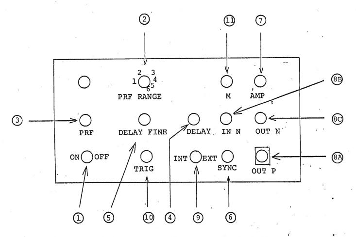
ON-OFF Switch. Applies basic prime power to all stages.
