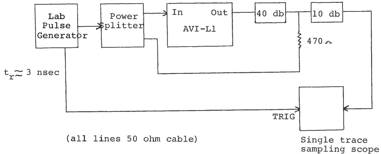
This arrangement allows the simultaneous display of the AVI-L1 input and output waveforms. No change of propagation delay could be detected when the PRF was varied over the range of about 20 Hz to 40 KHz (but it is to be noted that the 3 nsec rise time of the lab pulse generator output makes it relatively difficult to resolve extremely small propagation time variations).
