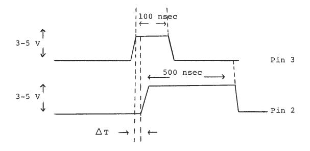
As the PW pot is varied over its full range  $\Delta T$  should vary from about 0 to approximately 100 nsec. If the waveforms at pins 2 and 3 do not resemble the above, then the -T module is defective and should be replaced. If the waveforms do resemble the above then the -PG module is at fault and should be replaced.
