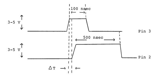
As the FW pot is varied over its full range  $\Delta$  T should vary from about 0 to approximately 100 nsec. If the waveforms at pins 2 and 3 do not resemble the above, then the -T module is defective and should be replaced. If the waveforms do resemble the above then the -PG module is at fault and should be replaced.
