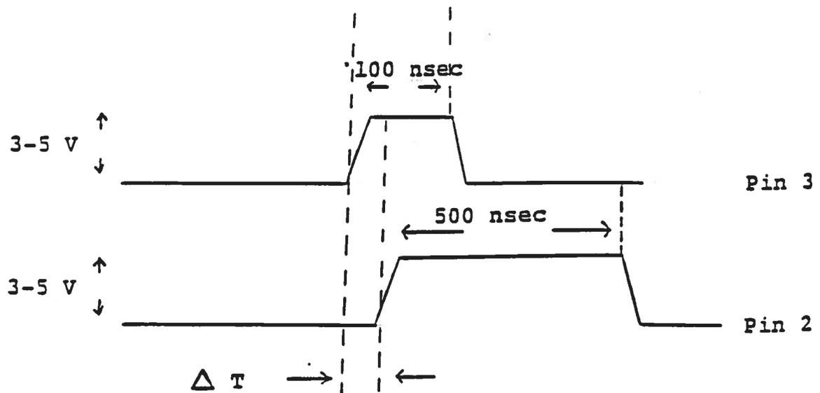
As the PW pot is varied over its full range  $\Delta T$  should vary from about 0 to approximately 100 ns. If the waveforms at pins 2 and 3 do not resemble the above, then the -T module is defective and should be replaced. If the waveforms do resemble the above then the -PG module is at fault and should be replaced.
