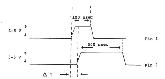
As the PW pot is varied over its full range  $\triangle$ T should vary from about 0 to approximately 100 ns. If the waveforms at pins 2 and 3 do not resemble the above, then the -T module is defective and should be replaced. If the waveforms do resemble the above then the -PG module is at fault and should be replaced.
