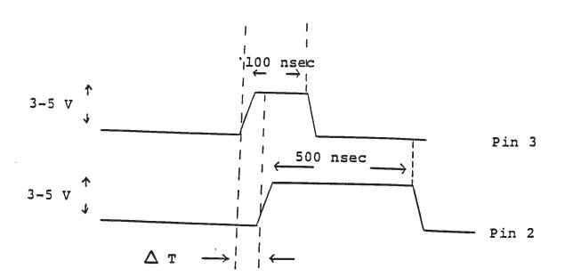
As the PW pot is varied over its full range  $\triangle$  T should vary from about 0 to approximately 100 ns. If the waveforms at pins 2 and 3 do not resemble the above, then the -T module is defective and should be replaced. If the waveforms do resemble the above then the -PG module is at fault and should be replaced.
