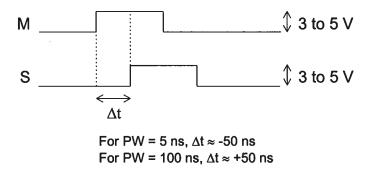
As the pulse width is varied over its full range ∆t should vary from about -50ns to approximately +50 ns. If the waveforms at the M and S pins do not resemble the above, then the -T101 module is defective and should be replaced. If the waveforms do resemble the above then the -PG module is at fault and should be replaced. Replacement modules should be ordered by part number (eg. AVL-2-PG) from Avtech.
