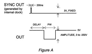
If the delay is negative, the order of the SYNC and OUT pulses is reversed:
