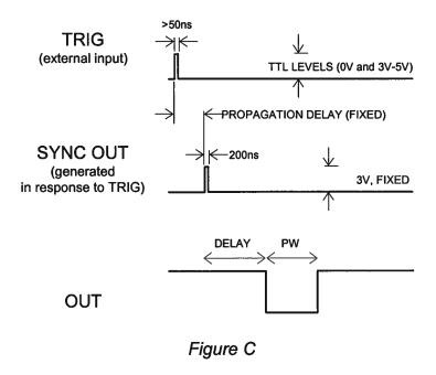
As before, if the delay is negative, the order of the SYNC and OUT pulses is reversed.
