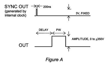
If the delay is negative, the order of the SYNC and OUT pulses is reversed:
