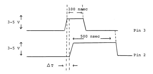
As the PW pot is varied over its full range  $\Delta$  T should vary from about 0 to approximately 100 ns. If the waveforms at pins 2 and 3 do not resemble the above, then the -T module is defective and should be replaced. If the waveforms do resemble the above then the -PG module is at fault and should be replaced.
