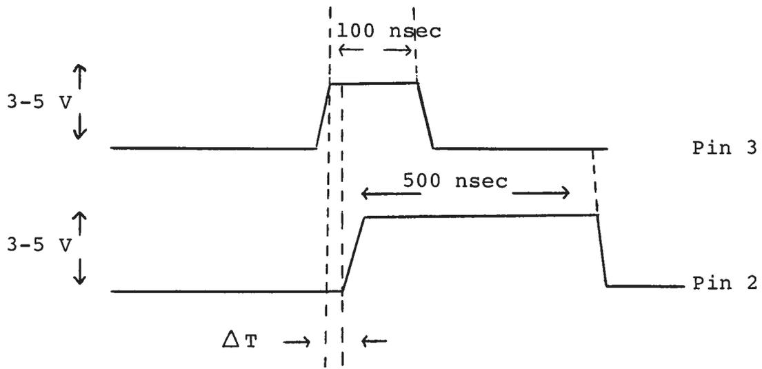
As the FW pot is varied over its full range  $\Delta T$  should vary from about 0 to approximately 100 nsec. If the waveforms at pins 2 and 3 do not resemble the above, then the -T module is defective and should be replaced. If the waveforms do resemble the above then the -PG module is at fault and should be replaced.
