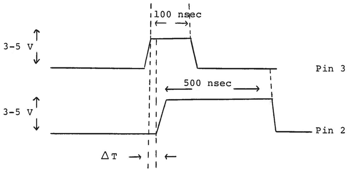
As the FW pot is varied over its full range  $\Delta T$  should vary from about 0 to approximately 100 nsec. If the waveforms at pins 2 and 3 do not resemble the above, then the -T module is defective and should be replaced. If the waveforms do resemble the above then the -FG module is at fault and should be replaced.
