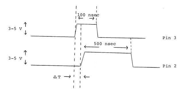
As the PW pot is varied over its full range T should vary from about 0 to approximately 100 nsec. If the waveforms at pins 2 and 3 do not resemble the above, then the -T module is defective and should be replaced. If the waveforms do resemble the above then the -PG module is at fault and should be replaced.
