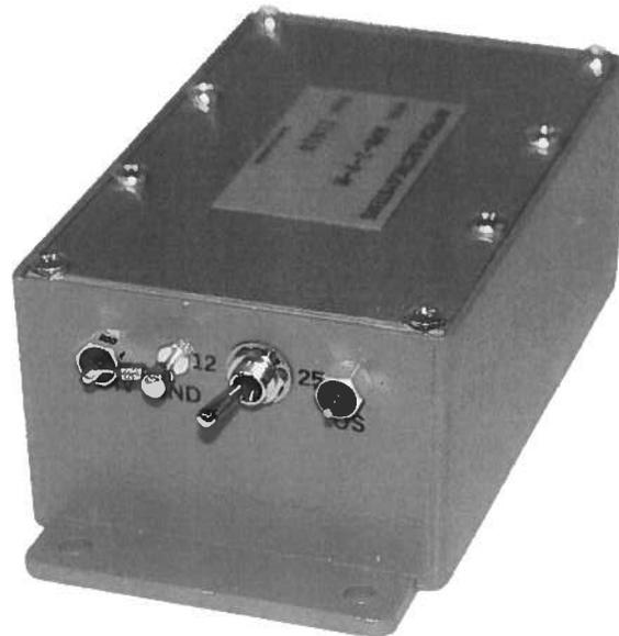
The “12/25” switch should be set in the “12” position if the PRF is less than 12 MHz. For higher PRF the switch should normally be in the “25” position for optimal rise times and pulse widths.
