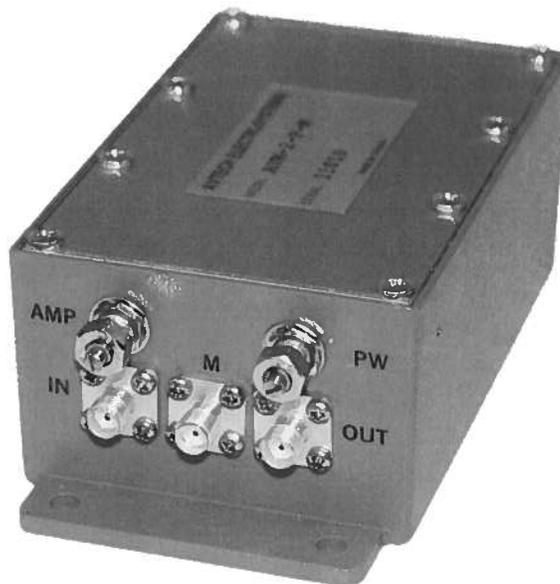
The “AMP” and “PW” controls may be adjusted using a screwdriver. Instruments with the -EA and -EW options will have solder terminal inputs to control the amplitude and pulse width, respectively, instead of screwdriver-adjustable controls. This is shown in the photo below:
