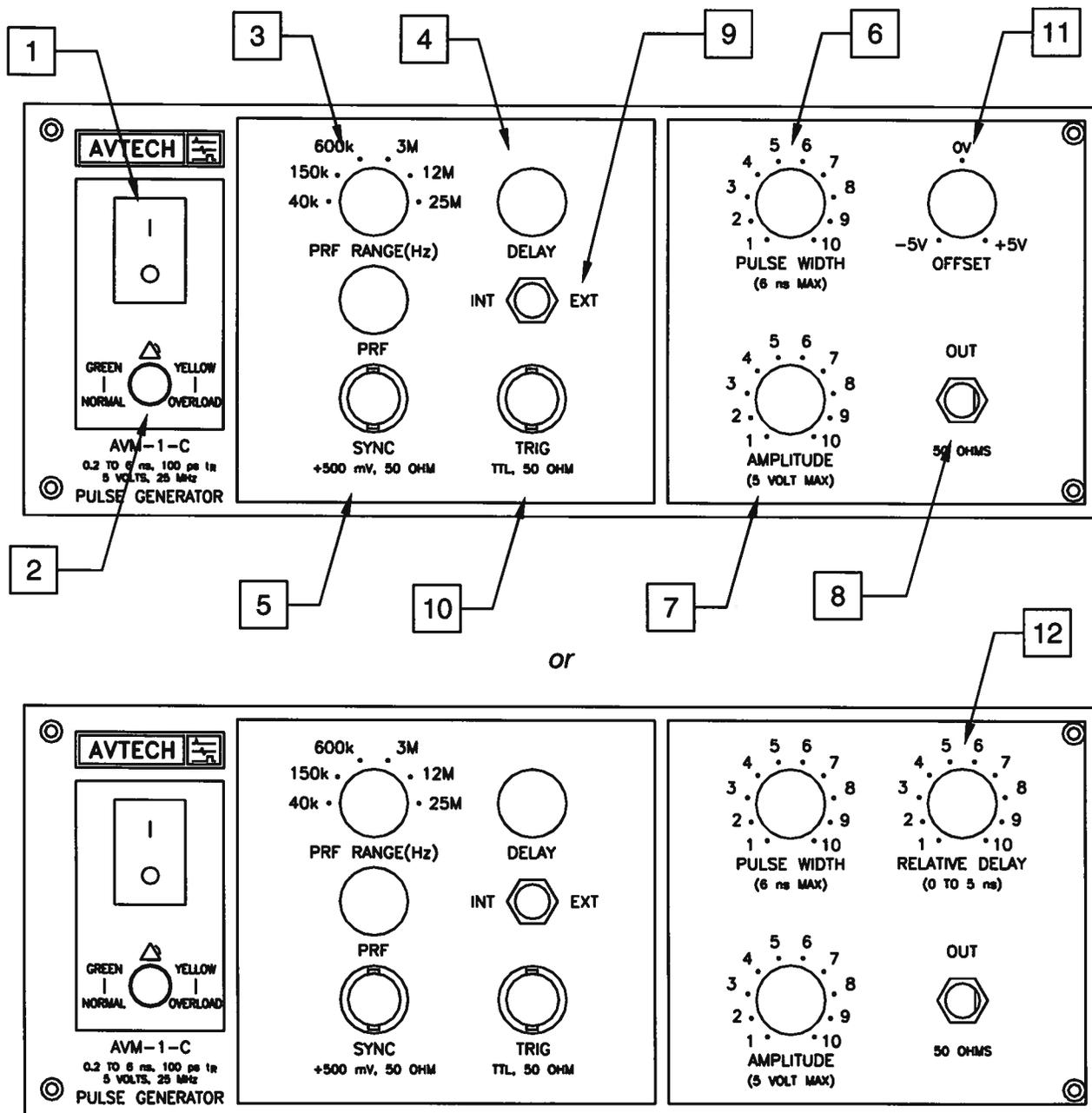
1. POWER Switch. This is the main power switch. When turning the instrument on, there may be a delay of several seconds before the instrument appears to respond.
