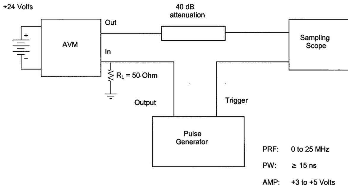
Power line: +24 Volts/0.50 Amps DC, shielded twisted pair, < 3 meters length
