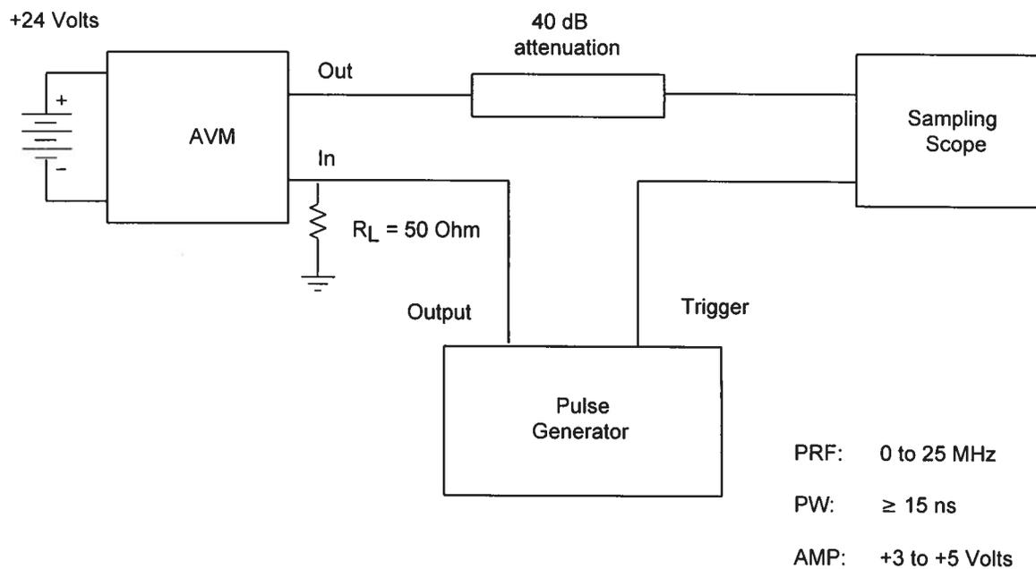
Power line: +24 Volts/0.50 Amps DC, shielded twisted pair, < 3 meters length
