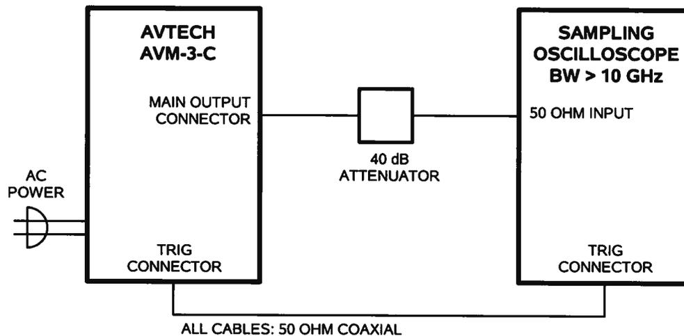
The attenuator is required to prevent damage to the sampling oscilloscope.
