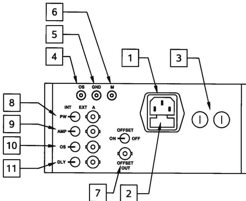
1. **AC POWER INPUT.** An IEC-320 C14 three-pronged recessed male socket is provided on the back panel for AC power connection to the instrument. One end of the detachable power cord that is supplied with the instrument plugs into this socket.
