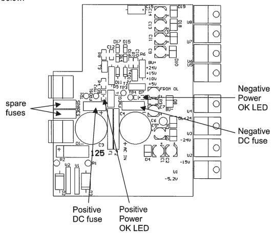
The positive fuse and one of the spare fuses on this circuit board are 1A slow-blow fuses, Littlefuse part number R452001. (This fuse can be ordered from Digikey, www.digikey.com. The Digikey part number is F1343CT-ND). The negative fuse and the second spare fuse are 0.5A slow-blow fuses (Littlefuse R452.500, Digikey part number F1341CT-ND).
