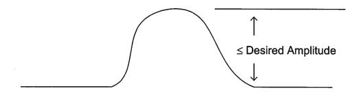
Having obtained a display of the form shown above, the desired pulse width is then obtained by adjusting the two front panel pots TR and TF. Rotate TR counter clockwise from the positive set in step 2) until a sharp 150 ps leading edge is observed. Then rotate TF counter-clockwise until the desired pulse width and fall time are obtained.
