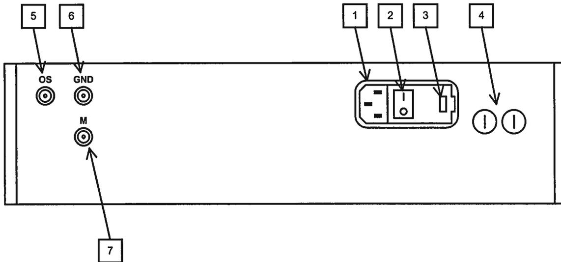
1. **AC POWER INPUT.** An IEC-320 three-pronged recessed male socket is provided on the back panel for AC power connection to the instrument. One end of the detachable power cord that is supplied with the instrument plugs into this socket.
