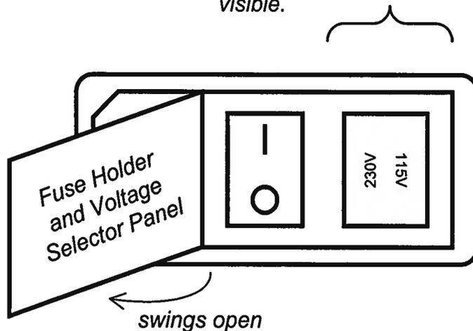
Once the panel is open, the red fuse holder / voltage selector should be visible. To change the voltage setting, pull out the red fuse holder / voltage selector and rotate it so that the proper voltage marking will shown through the panel window. Re-install the red fuse holder / voltage selector, and close the panel.
