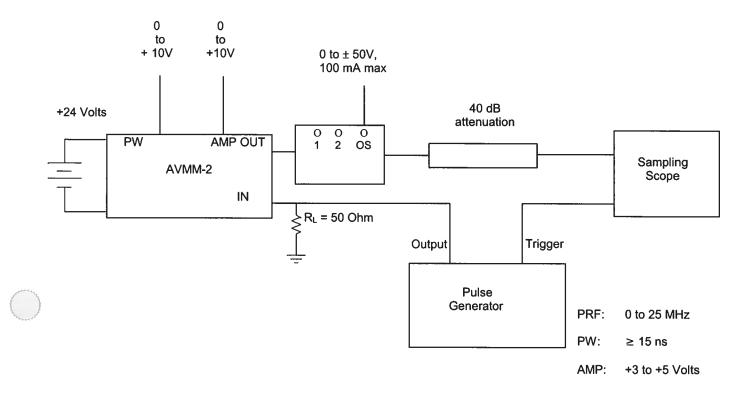
Power Line:+24 Volts / 0.5 Amps DC, shielded twisted pair, < 3 meters length</td>Control Lines:1 – Coaxial line, (trigger), SMA connector, < 3 meters length</td>1 – Shielded twisted pair, (offset), < 3 meters length</th>1 – Shielded twisted pair, (EW), < 3 meters length</th>Output:Coaxial, SMA, < 3 meters length</td>
