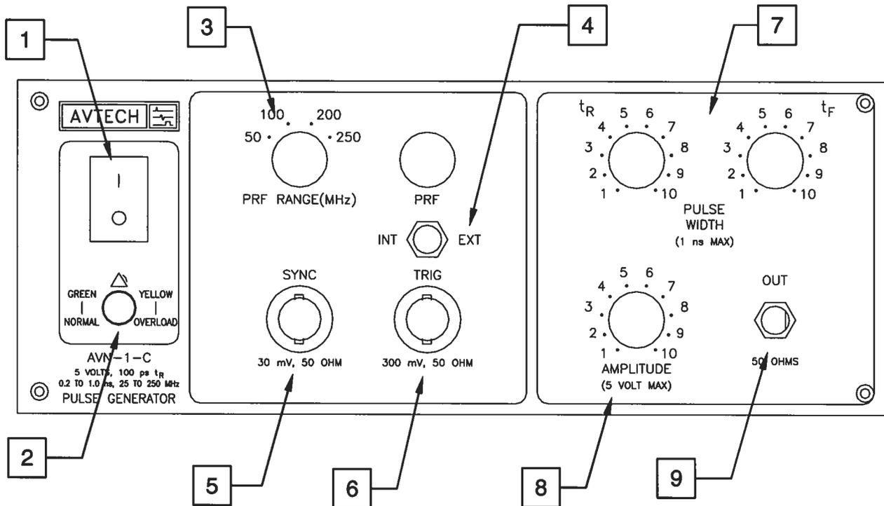
1. **POWER Switch**. This is the main power switch. When turning the instrument on, there may be a delay of several seconds before the instrument appears to respond.
