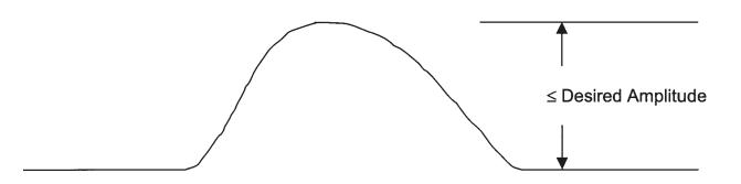
5) Having obtained a display of the form shown above, the desired pulse width is then obtained by adjusting the two front panel pots TR and TF. Rotate TR counter clockwise from the positive set in step 2) until a sharp 100 ps leading edge is observed. Then rotate TF counterclockwise until the desired pulse width and fall time are obtained.
