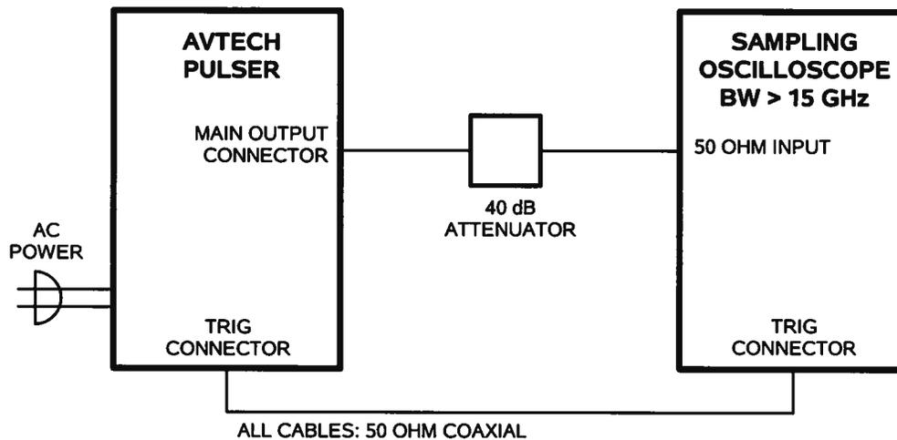
The attenuators are required to prevent damage to the sampling oscilloscope. A 40 dB attenuator with sufficient voltage rating should be used on the main output.
