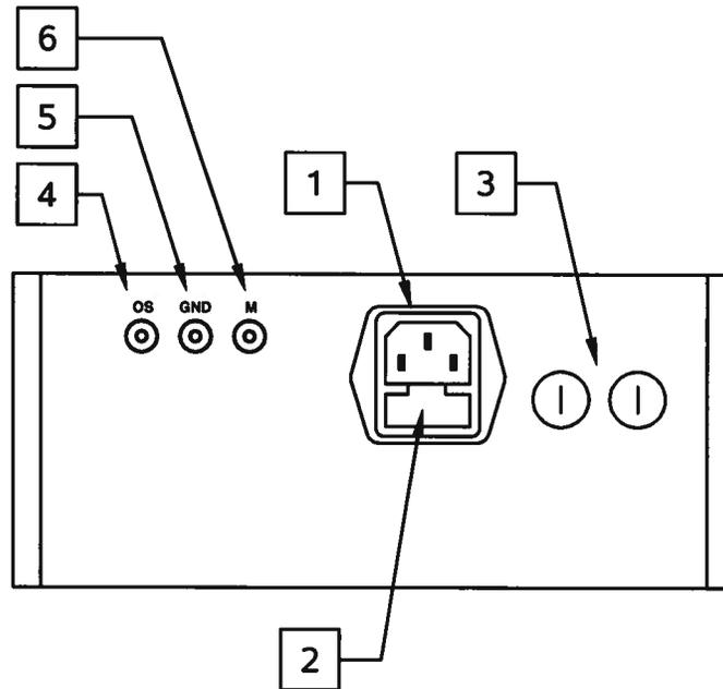
1. **AC POWER INPUT.** An IEC-320 C14 three-pronged recessed male socket is provided on the back panel for AC power connection to the instrument. One end of the detachable power cord that is supplied with the instrument plugs into this socket.
