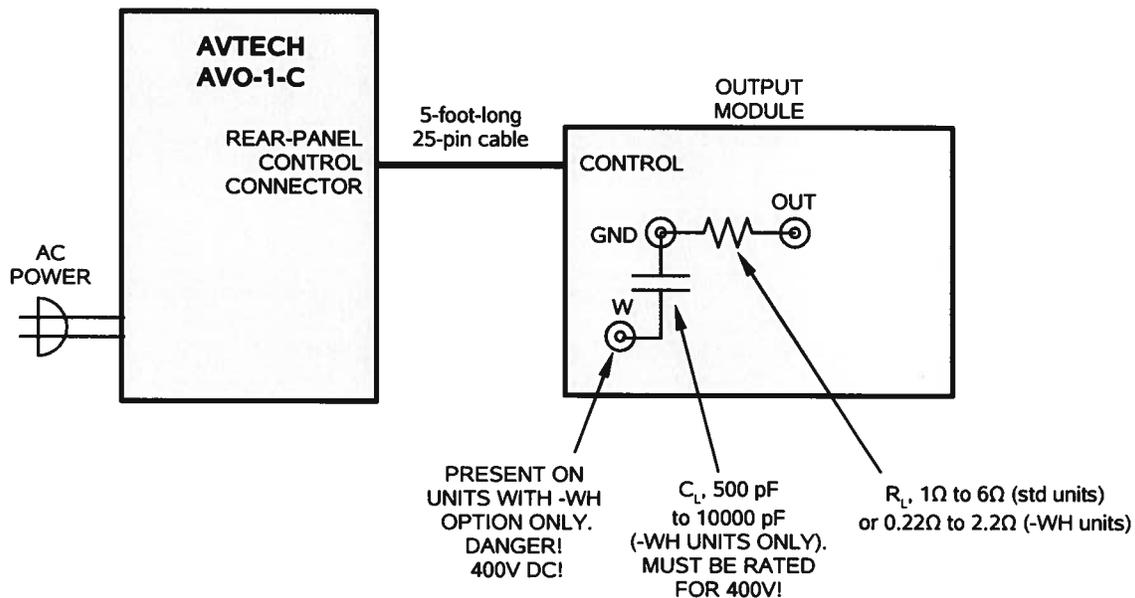
To access the OUT, GND, and W (for -WH units) terminals, the aluminum cover plate must be removed, by unscrewing it from the bottom of the output module. The unit must be turned off and unplugged when the cover plate is removed.
