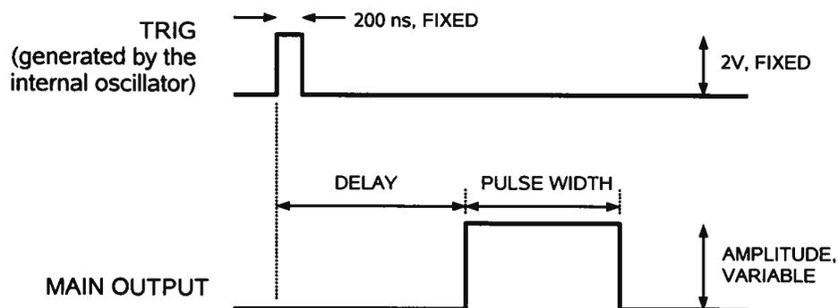
When the ADVANCE/DELAY switch is set to "DELAY", the TRIG output occurs after the main output. This is illustrated below:
