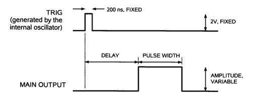
When the ADVANCE/DELAY switch is set to "DELAY", the TRIG output occurs after the main output. This illustrated below:
