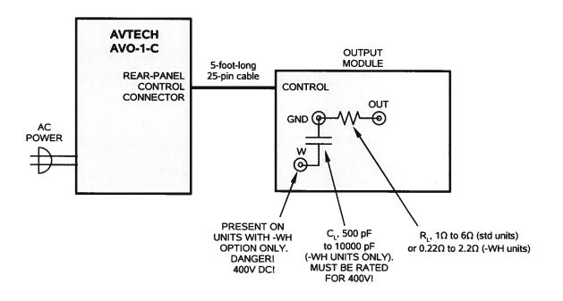
To access the OUT, GND, and W (for -WH units) terminals, the aluminum cover plate must be removed, by unscrewing it from the bottom of the output module. The unit must be turned off and unplugged when the cover plate is removed.
