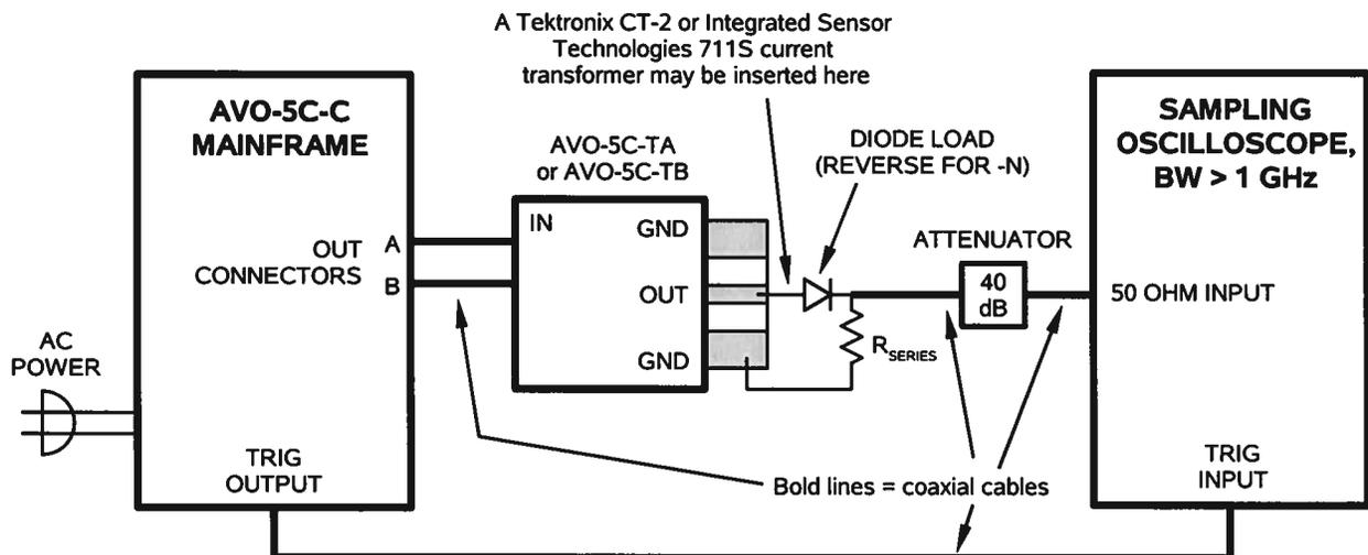
The attenuator is required to prevent damage to the sampling oscilloscope.
