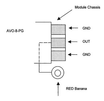
The load should be connected between the OUT and GND terminals using very short leads ( $\leq 2.0$  cm).
