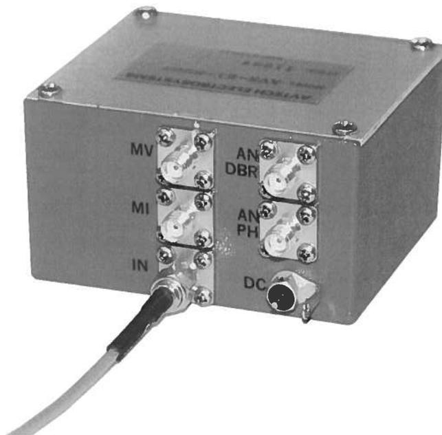
An oscilloscope may be used to monitor the MI and MD outputs, the locations of which are shown in the figure above. A forward DC bias may be applied to the laser diode by connecting a DC potential of 0 to +5 Volts to the DC solder terminal. The application of a small forward bias often yields a more ideal diode current waveform (as observed on the MI port). Note that the DC port must be shorted to ground if a bias is not applied.
