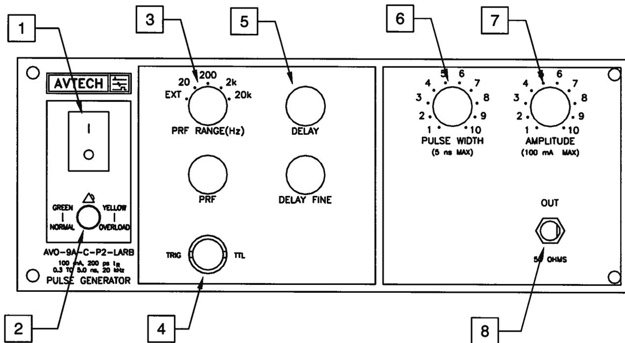
1. **POWER Switch.** This is the main power switch. When turning the instrument on, there may be a delay of several seconds before the instrument appears to respond.
