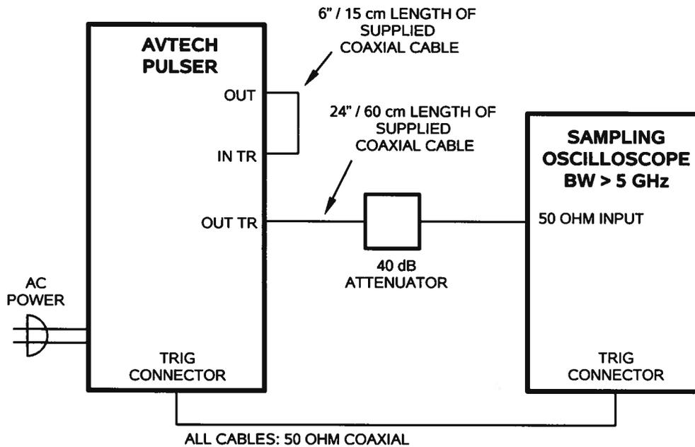
The attenuators are required to prevent damage to the sampling oscilloscope. A 40 dB attenuator with sufficient voltage rating should be used on the main output.
