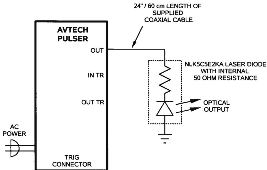
When connecting to the diode, care must be taken to maintain a proper high-bandwidth 50 Ohm transmission line system, using high-speed construction techniques.
