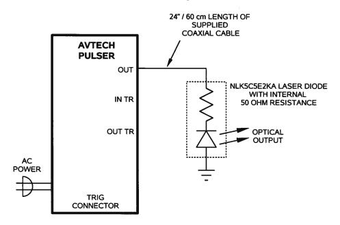
When connecting to the diode, care must be taken to maintain a proper high-bandwidth 50 Ohm transmission line system, using high-speed construction techniques.
