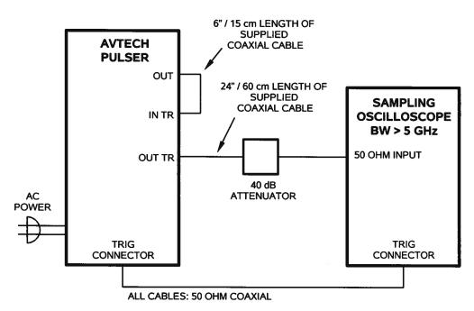
The attenuators are required to prevent damage to the sampling oscilloscope. A 40 dB attenuator with sufficient voltage rating should be used on the main output.
