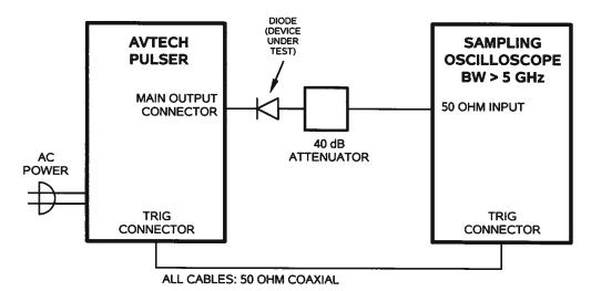
In this setup, the attenuator and the oscilloscope act as the  $50\Omega$  resistance in series with the diode. When connecting to the diode, care must be taken to maintain a proper
