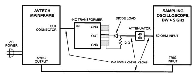
The lead lengths on the output side of the transformer must be kept extremely short (a few millimeters) to maintain high-speed operation.
