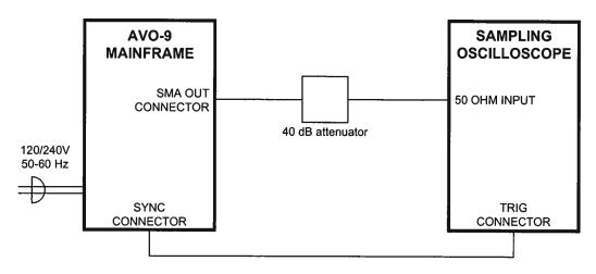
Since most sampling oscilloscopes have limited input amplitude ranges, an attenuator on the AVO-9 output is normally required.
