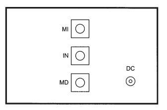
AVX-S1-HC OUTPUT MODULE, CONNECTOR VIEW
