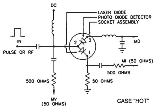
Fig. 2 - AVX-S1 and AVX-S2 functional equivalent circuit (alternative configuration)
