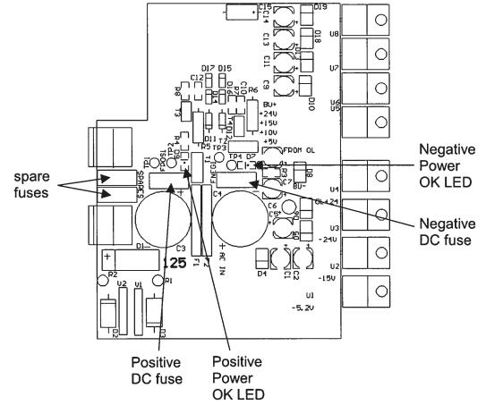
The positive fuse and one of the spare fuses on this circuit board are 1A slow-blow fuses, Littlefuse part number R452001. (This fuse can be ordered from Digikey, www.digikey.com. The Digikey part number is F1343CT-ND). The negative fuse and the second spare fuse are 0.5A slow-blow fuses (Littlefuse R452.500, Digikey part number F1341CT-ND).
