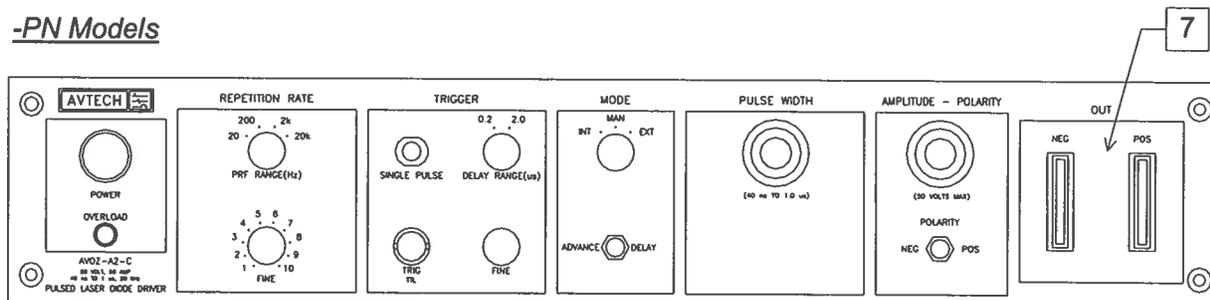
1. **POWER Switch.** The POWER push button switch applies AC prime power to the primaries of the transformer, turning the instrument on. The push button lamp (#382 type) is connected to the internal +15V DC supply.
