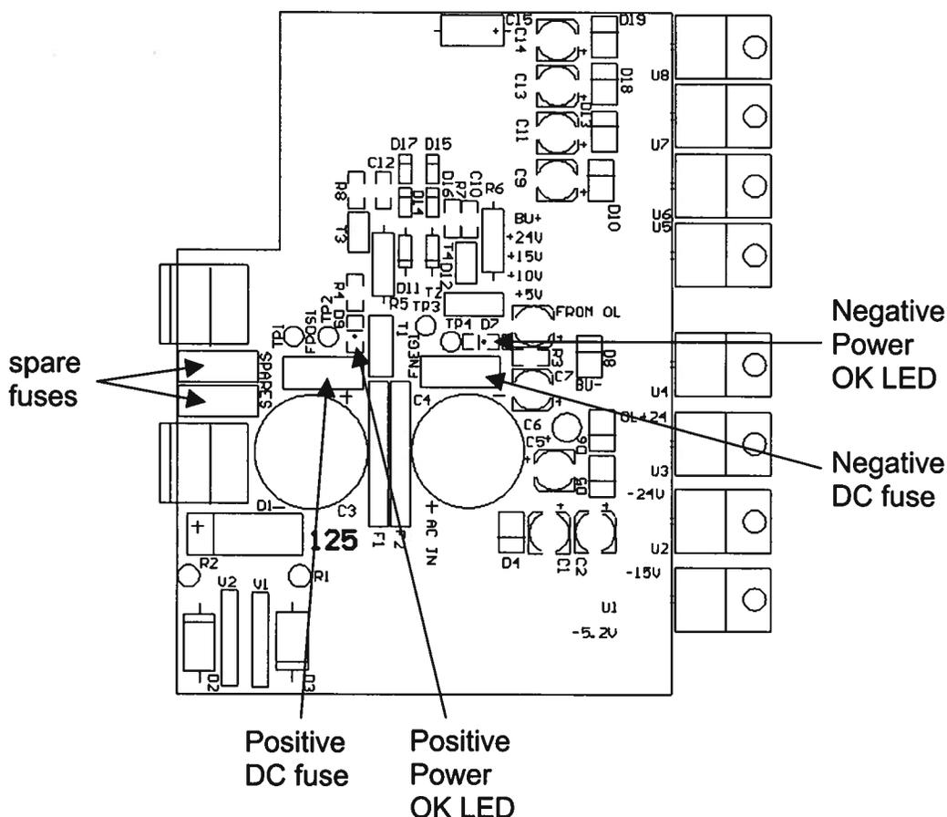
The positive fuse and one of the spare fuses on this circuit board are 1.5A slow-blow fuses, Littlefuse part number R45201.5. (This fuse can be ordered from Digikey, [www.digikey.com](http://www.digikey.com). The Digikey part number is F1344CT-ND). The negative fuse and the second spare fuse are 0.5A slow-blow fuses (Littlefuse R452.500, Digikey part number F1341CT-ND).
